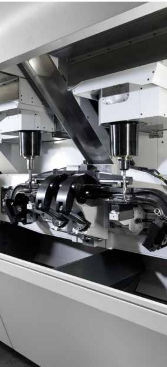
The UNITWIN 6000 is equipped with two very powerful main spindles. Both of them can tilt up to plus and minus 15 degrees, so they can handle all operations on the various king pin angles available in the market. The two spindles work simultaneously to finish front axles in the quickest possible time for a major reduction in cycle times. These can be as little as 4,5 minutes per axle.
