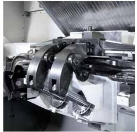
One further strong point of the UNISIGN front axle machining solutions is their flexibility. With minimum effort, the fixture can be altered to allow a large variety of front axles to be clamped. There is even an option to change the full fixture, which allows customers to produce less common types of beams, such as bus front axles.
